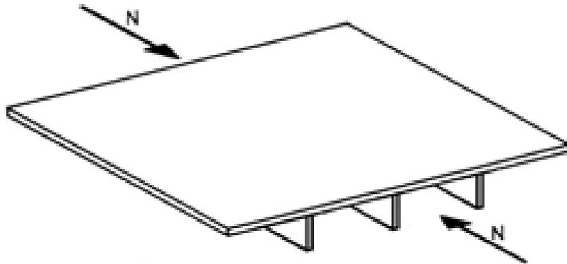
**Fig. 1.** Longitudinally stiffened plate loaded by uniaxial compression
