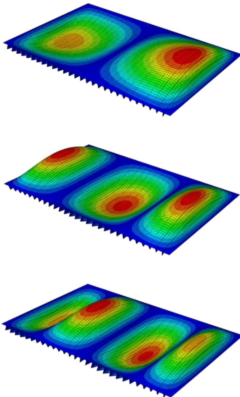
**Fig. 2.** The first four modes of vibrations of rectangular plate
