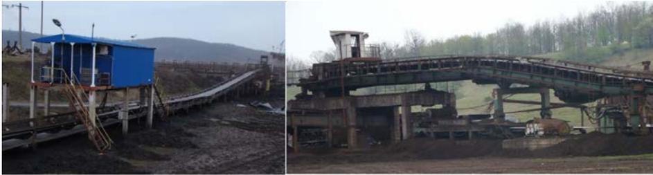
Fig. 1. High capacity conveyer belt with a mobile/non-stationary delivery end.
