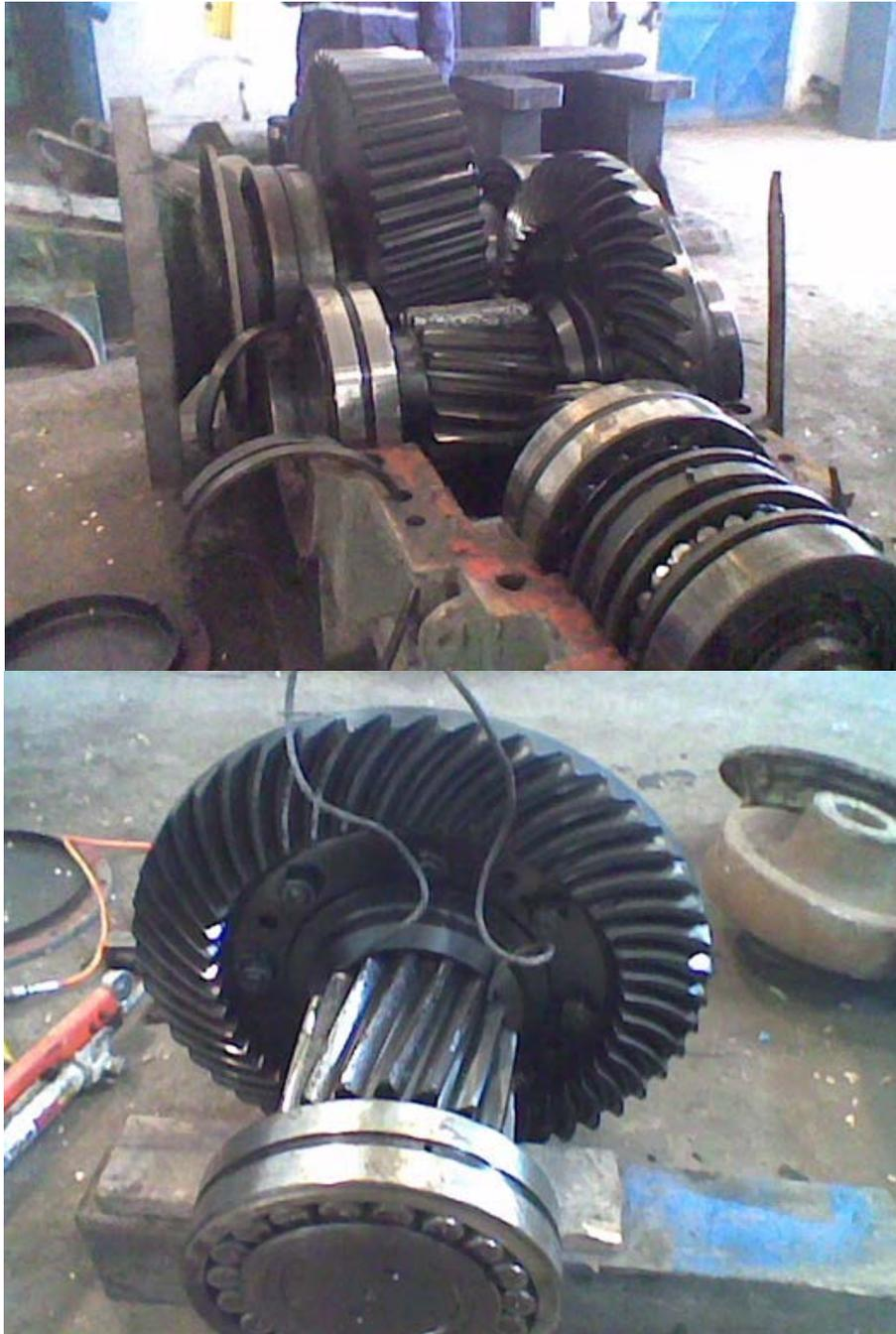
**Fig. 7.** The wearing mode of the tothing of the reducer 2KC-P-630
