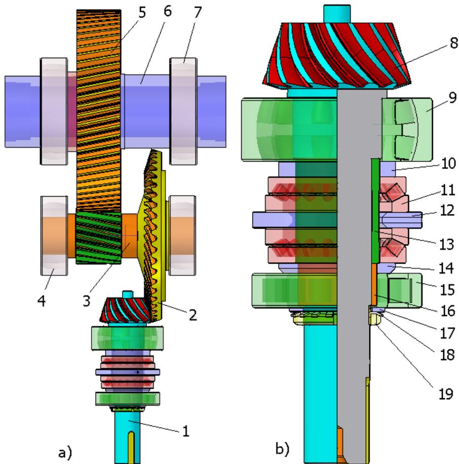
**Fig. 6.** 3D model of the transmission of the reducer
