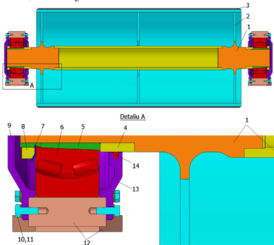
Fig. 5. 3D model of the free enhanced drum
