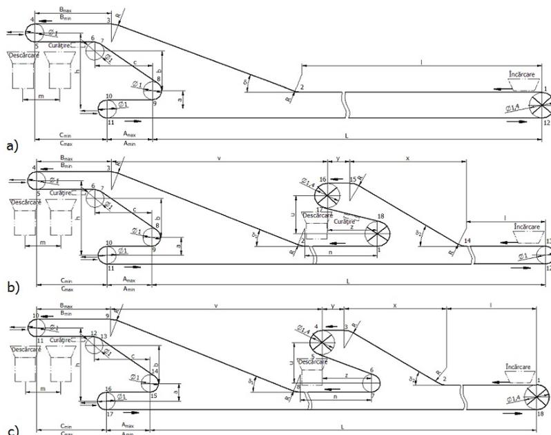
Fig. 2. The outline of the conveyer belt in its three constructive variants.
