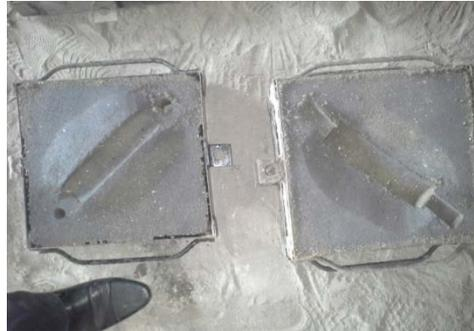
Fig. 2. Prepared mould for one of the cylindrical shapes
