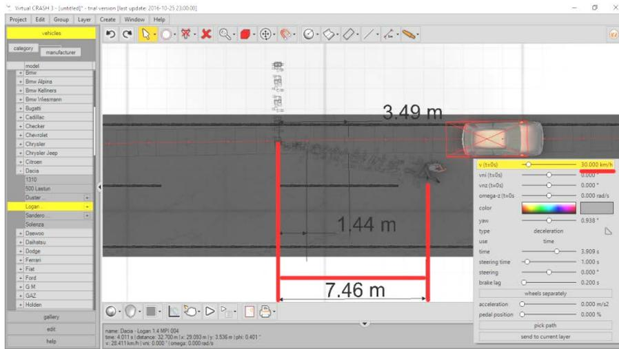
Fig. 6 Details of the simulation for 30 km/h with measured distance
