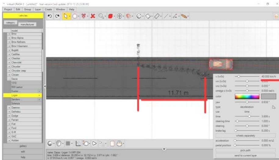
Fig. 7 Details of the simulation for 40 km/h with measured distance
