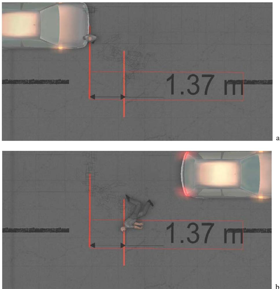
**Fig. 4** Details of the simulation for 10 km/h with measured distance
