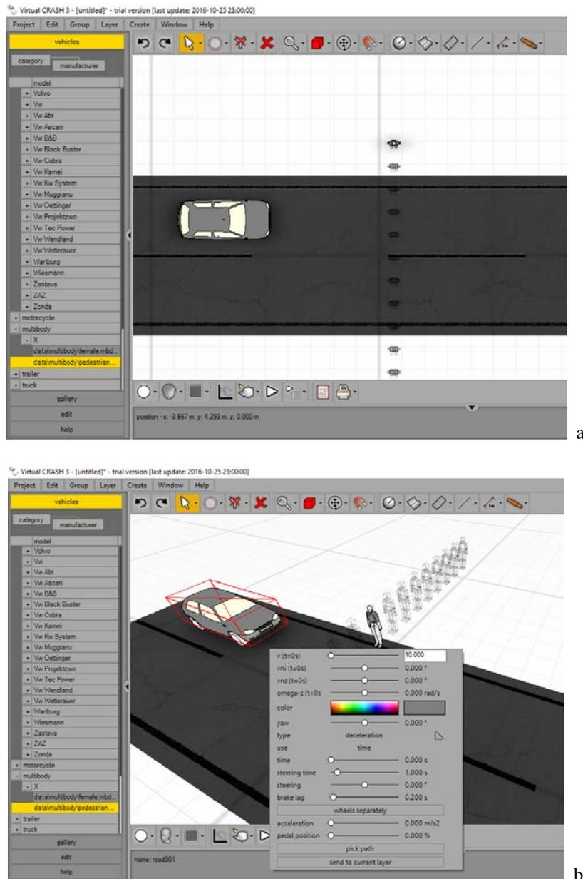
**Fig. 3** Model of accident: a) 2D view; b) 3D view and vehicle speed setup
