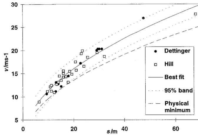
**Fig. 1.** Pedestrian throw distance and vehicle speed for Hill and Dettinger. (Source [6])
