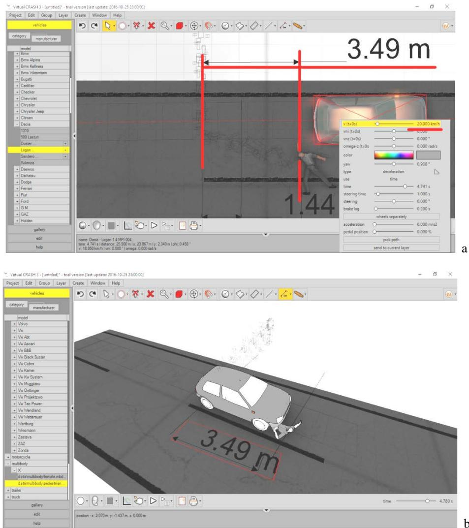
**Fig. 5** Details of the simulation for 20 km/h with measured distance
