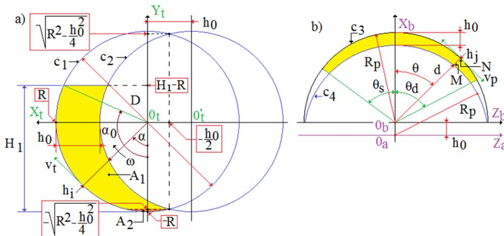
Fig. 2. The parameters of the cutting process.
