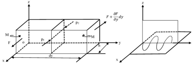
**Fig. 2.** Graphical representation of the forces occurring in a homogeneous plate
