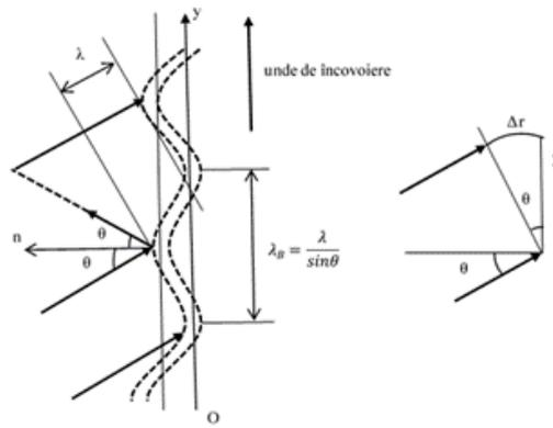
Fig. 3. Transmission of bending wave in a homogeneous plate
