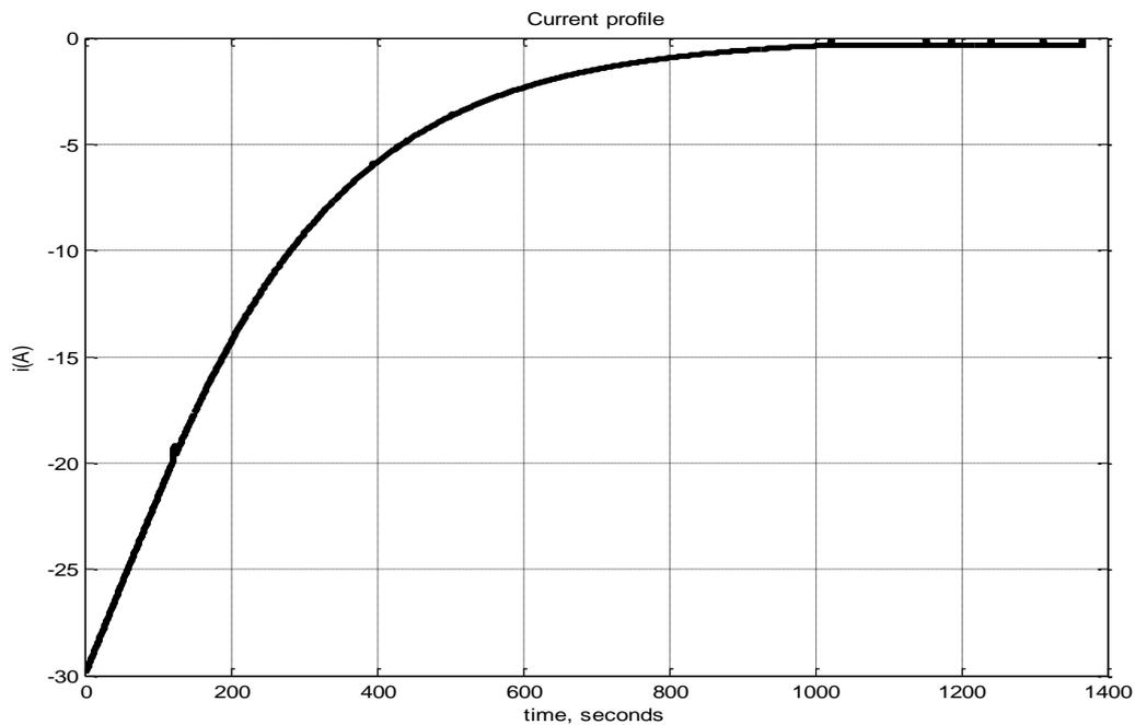
Fig. 2. The ADVISOR EPA UDDS current driving cycle profile
