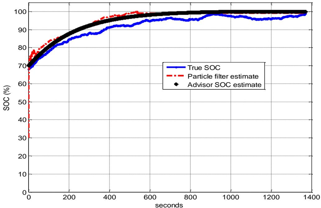
Fig. 6. The Robustness of PKF estimator to the changes in SOC initial value
