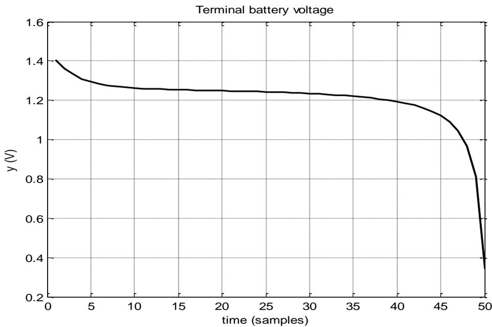
**Fig. 1.** The Ni-MH battery OCV discharging curve
