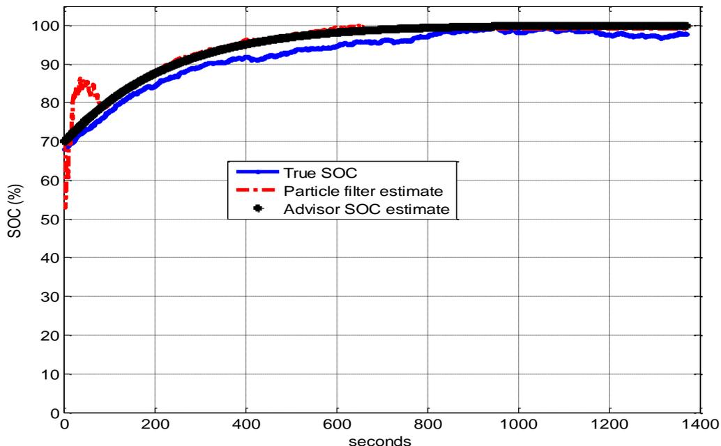
Fig. 3. The Battery SOC estimated by PKF estimator
