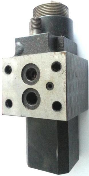
Fig. 4. The disconnection valve prototype.
