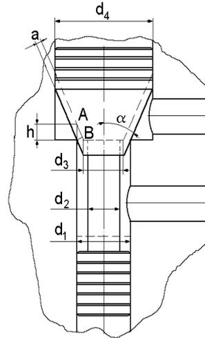
Fig. 5. The valve calculation scheme.
