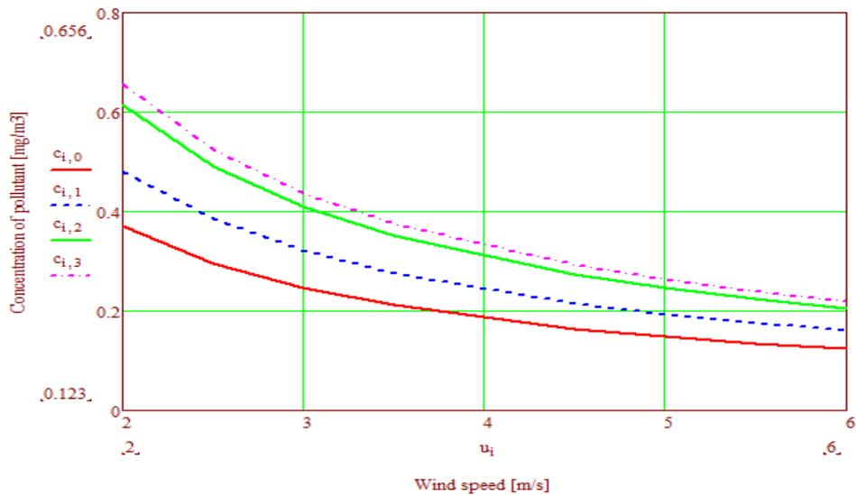
**Fig. 3.** Function  $c = f(u, \dot{m})$ , considering the values of the variable wind speed and the constant mass flow
