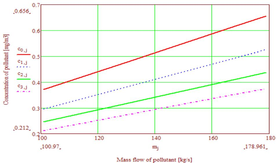
**Fig. 4.** Function  $c = f(u, \dot{m})$ , considering the values of a constant wind speed and a variable mass flow
