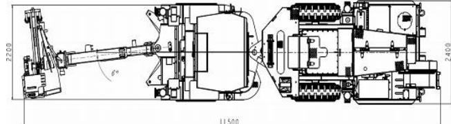
**Fig. 10.** Model of the designed solution of a roof bolter with the values of its maximum width and length, with the jib and the turret being turned by 6°
