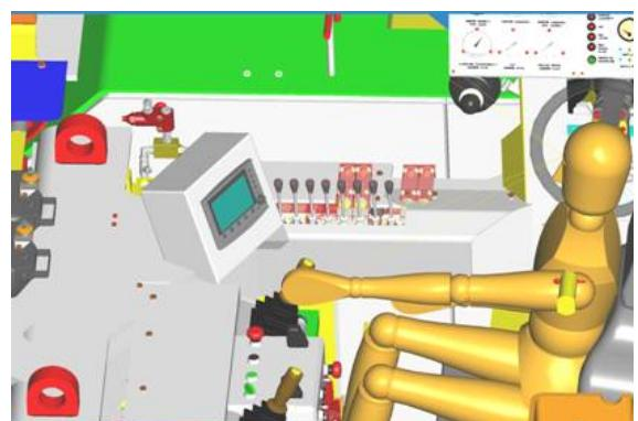
**Fig. 14.** Result of a simulation of the operator's access to the control desk during the drilling-bolting processes in terms of ergonomics of the operator's work during operation in the mine face
