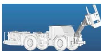
**Fig. 9.** Spatial model of a preliminary design of a new solution of a roof bolter for medium layers – side view
