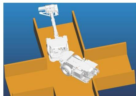
**Fig. 13.** Simulation of a ride in dog headings intersecting at an angle of 90° without a need to cut off the corners
