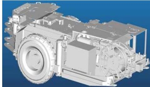
**Fig. 6.** Spatial model of a preliminary design of a tractor of a new solution of a roof bolter for medium layers. A view from the back, left hand side
