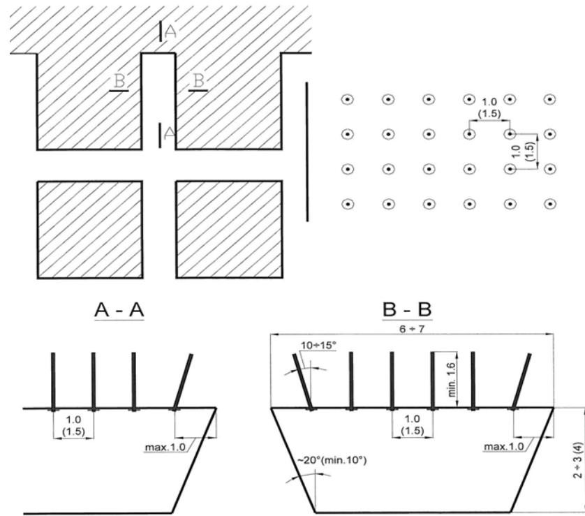
**Fig. 3.** Diagram of a working network along with a suggested bolting net and longitudinal and cross sections of a dog heading
