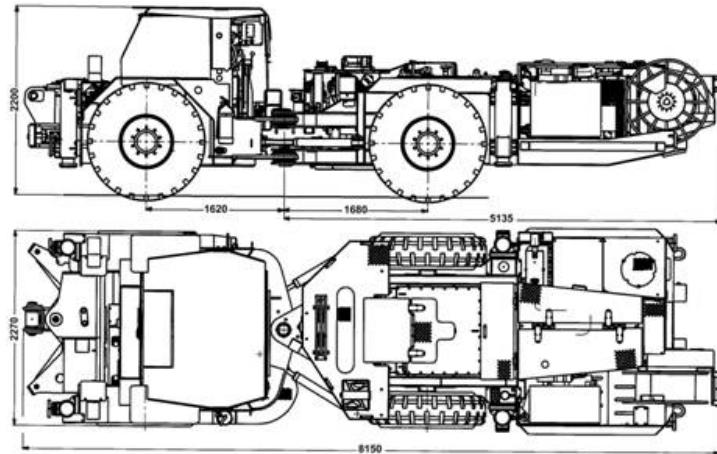
**Fig. 8.** Preliminary design of a chassis and bodywork a new solution of a roof bolter for medium layers, overall dimensions
