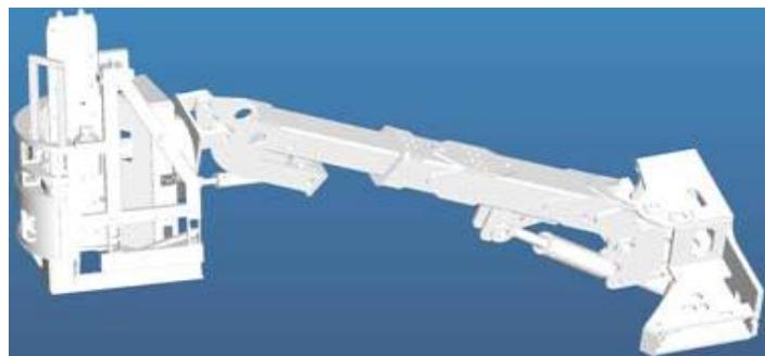
**Fig. 5.** Spatial model of the preliminary design of a working system of a new solution of a roof bolter for medium layers
