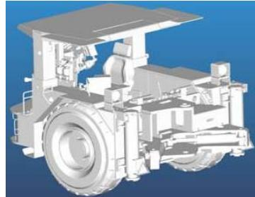
**Fig. 7.** Spatial model of a preliminary design of a working platform of a new solution of a roof bolter for medium layers. A view from the front of the driver's cabin
