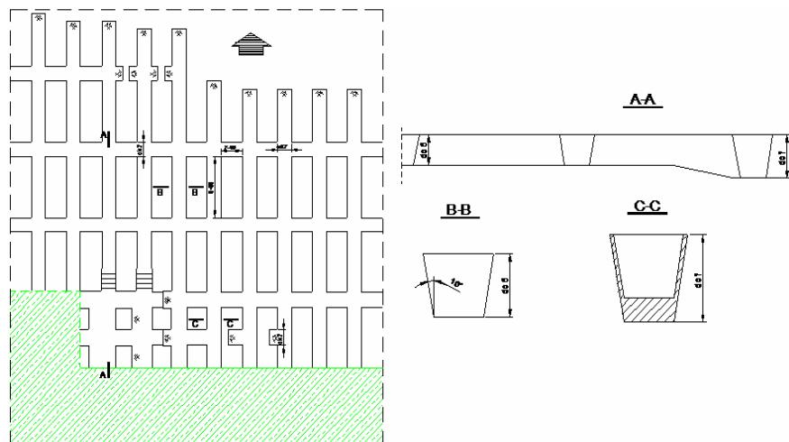
**Fig. 2.** Diagram of exploitation by the room and pillar system with susceptibility of deposit and additional roof protection
