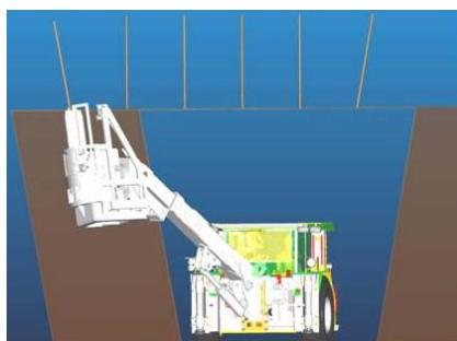
**Fig. 12.** Result of a simulation of an installation of bolts near the right sidewall
