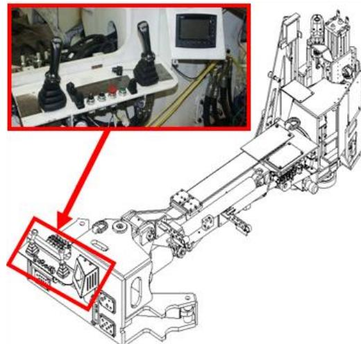
**Fig. 11.** Position of joysticks for controlling the jib, rotations and the feed on the control desk in the operator's cabin
