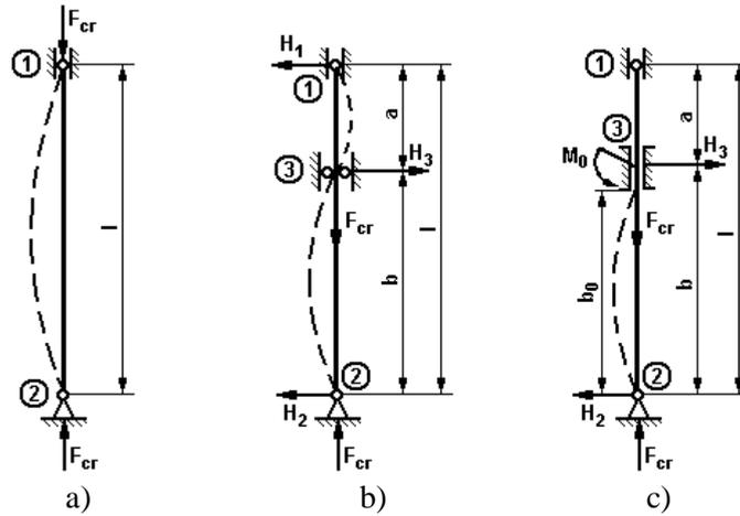
Fig. 4. Calculation patterns for the rack
