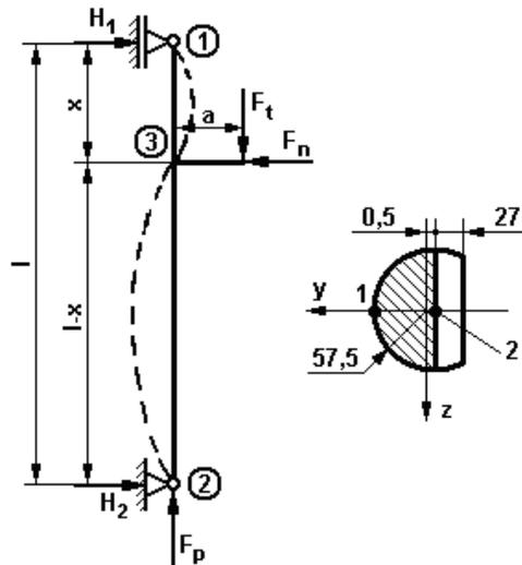
Fig. 3. Calculation pattern for the rack
