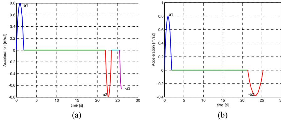
**Fig. 4.** Variation of acceleration in the case of parabolic speed modeling, with speed step (a) and with continuous speed (b)
