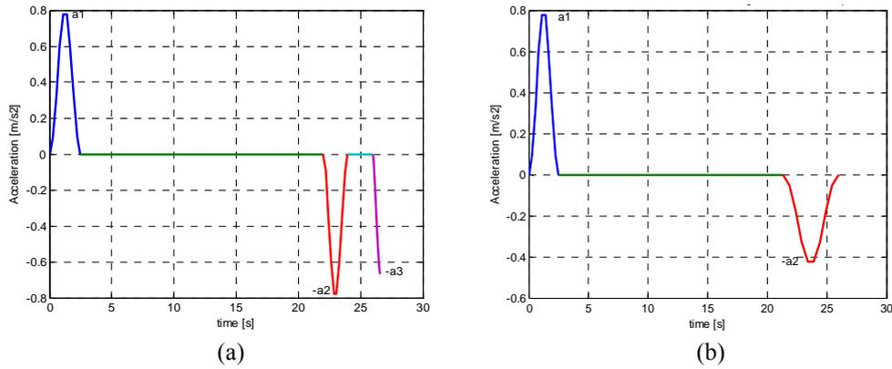
**Fig. 7.** Variation of acceleration in the case of cosinusoidal speed modeling, with speed step (a) and with continuous speed (b)
