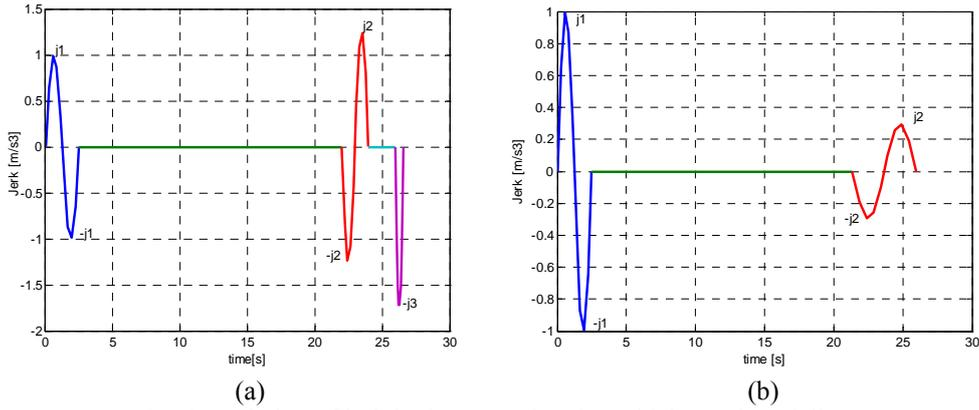
**Fig. 6.** Variation of jerk in the case of cosinusoidal speed modeling, with speed step (a) and with continuous speed (b)
