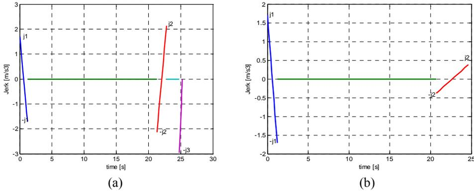
**Fig. 3.** Variation of jerk in the case of parabolic speed modeling, with speed step (a) and with continuous speed (b)
