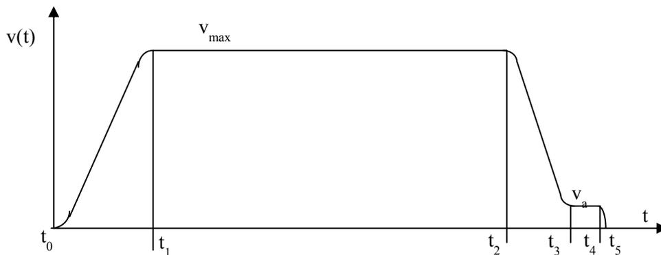
**Fig. 1.** Time periods of a functioning cycle for an elevator with constant speed step deceleration
