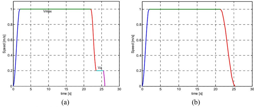
**Fig. 5.** Variation of speed in the case of parabolic speed modeling, with speed step (a) and with continuous speed (b)
