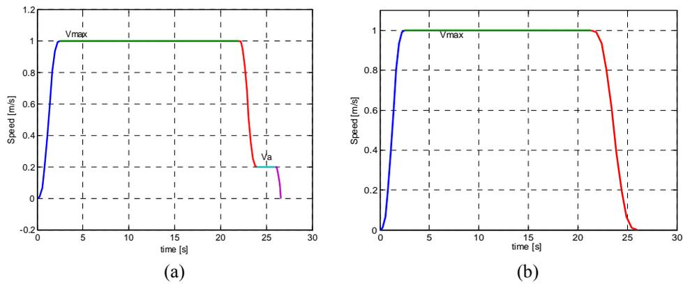
**Fig. 8.** Variation of speed in the case of cosinusoidal speed modeling, with speed step (a) and with continuous speed (b)
