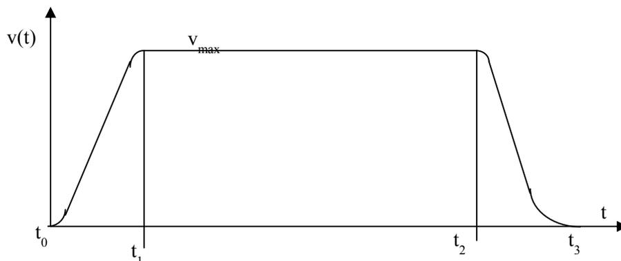
**Fig. 2.** Time periods of a functioning cycle for an elevator with continuous speed deceleration
