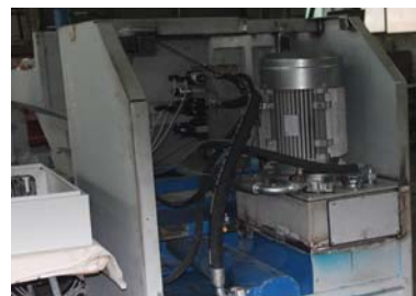
Fig. 11. Electric-hydraulic group with command block and pressing cylinder
