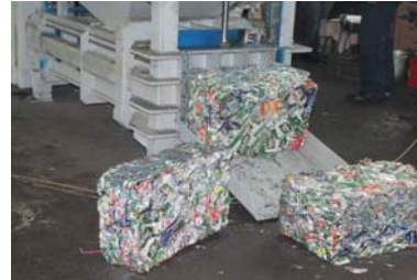
Fig. 13. Way of exhaust of bale from aluminum doses
