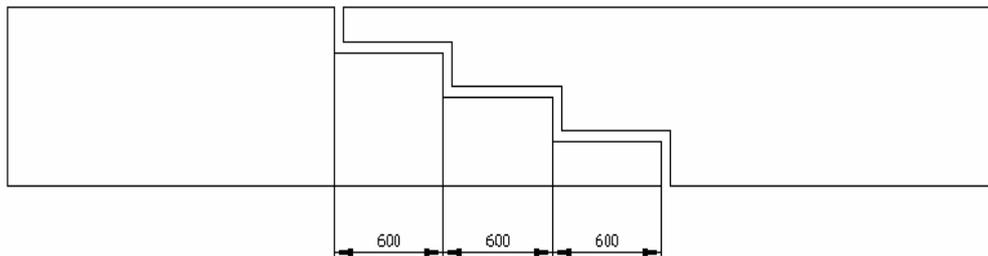
**Fig. 1.** One way of preparing the conveyor belt ends
