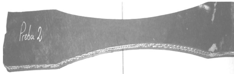
**Fig. 3.** Form tensile specimen tested
