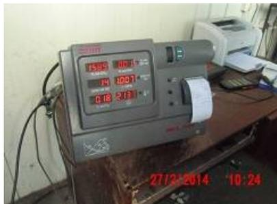
Fig. 9. Accelerated idle run measurements
