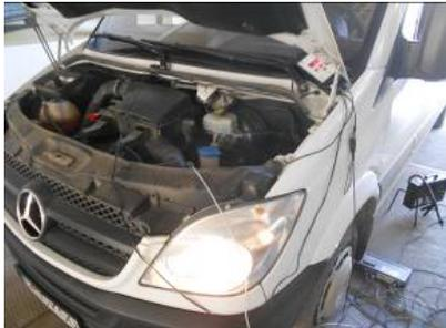
Fig. 7. Placing the measurement sensors
