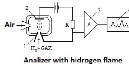
**Fig. 3.** Hydrogen flame analyzer
