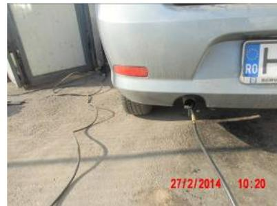
Fig. 10. Exhaust fumes measurement sensor
