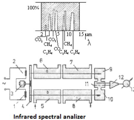
**Fig. 2.** Infrared radiation spectral analyzer
