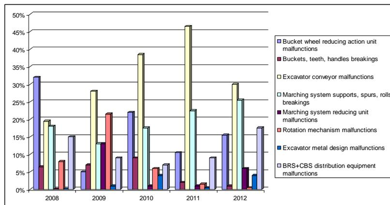
Fig. 10. Shares of various mechanical interruptions among excavator mechanical interruptions
