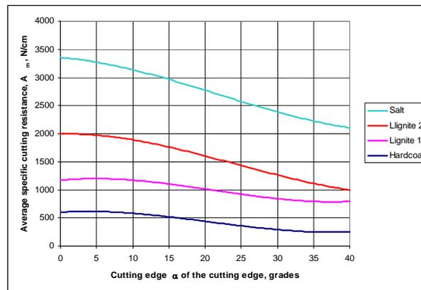
Fig. 8. Dependence of average cutting resistance  $A_m$  on raking angle  $\alpha$
