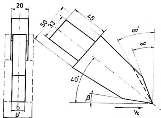
Fig. 3. Layout of test bits; realization of the test bit kit
