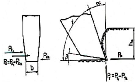
Fig. 7. Main parameters of the bit and cut
