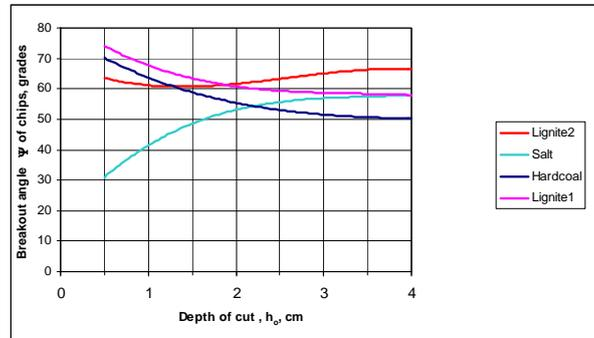
Fig. 9. Breakout angle  $\Psi$  dependence on depth of cut  $h_o$
