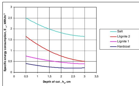
Fig. 10. The variation of specific energy consumption in respect with the depth of cut
