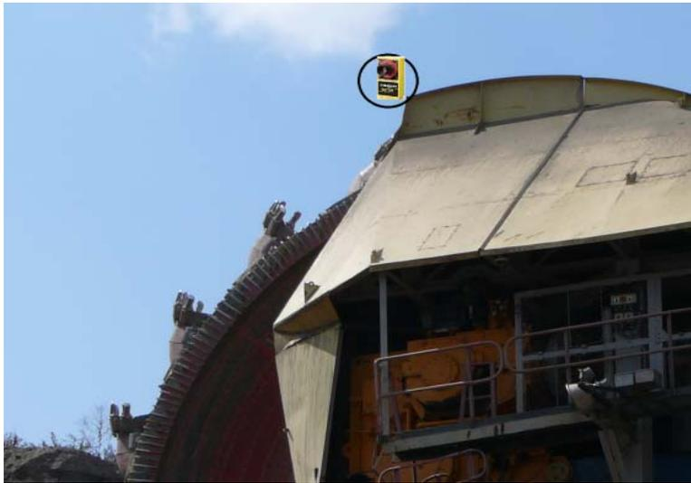
**Fig. 4.** DVT Vision sensor position on the bucket wheel excavator
