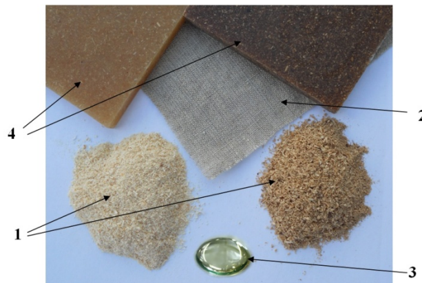
Fig.5. Material composition: 1 - wood flour (oak and spruce species); 2 - weave fabric of flax fibres; 3 - epoxy resin; 4 –composite materials
