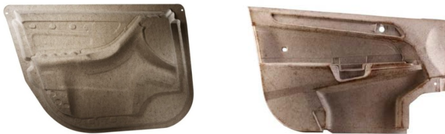
Fig.4. Carriers for covered door panels made of natural fibres with polymer resin [6]
