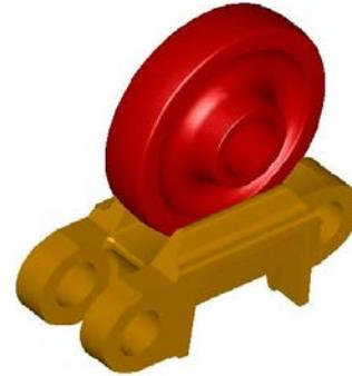
**Fig. 2.** 3D model of the caterpillar track body-roller system
