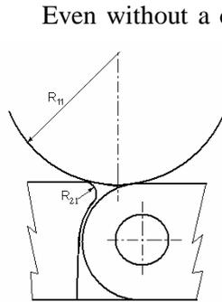
**Fig.6.** Relative locations of the roller and the bases, in an intermediate position
