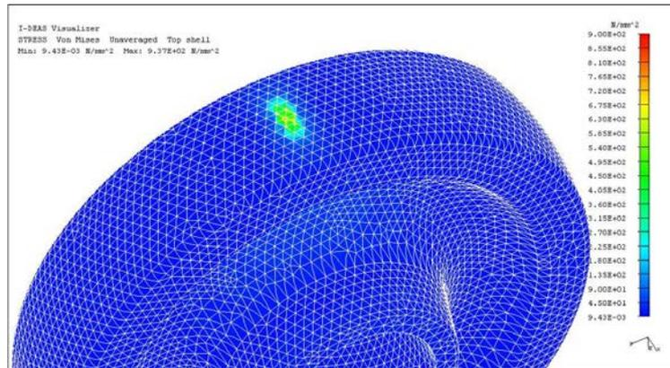
**Fig. 5.** FEM discretization of the roller
