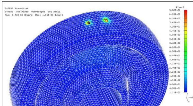
**Fig. 8.** Stress state resulted from FEM modeling showing the 2 stress peak zones
