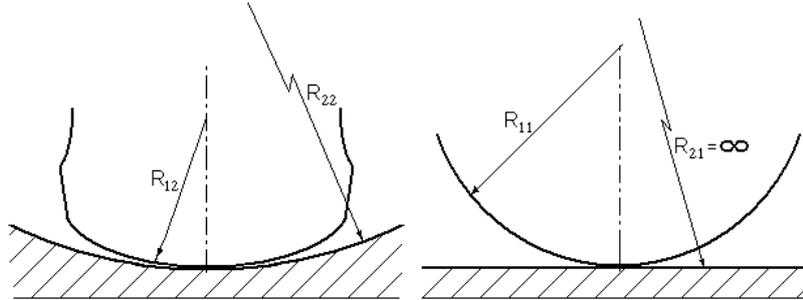
Fig. 4. Curvature radii of the contact zone. Cross section(left) longitudinal profile(right)
