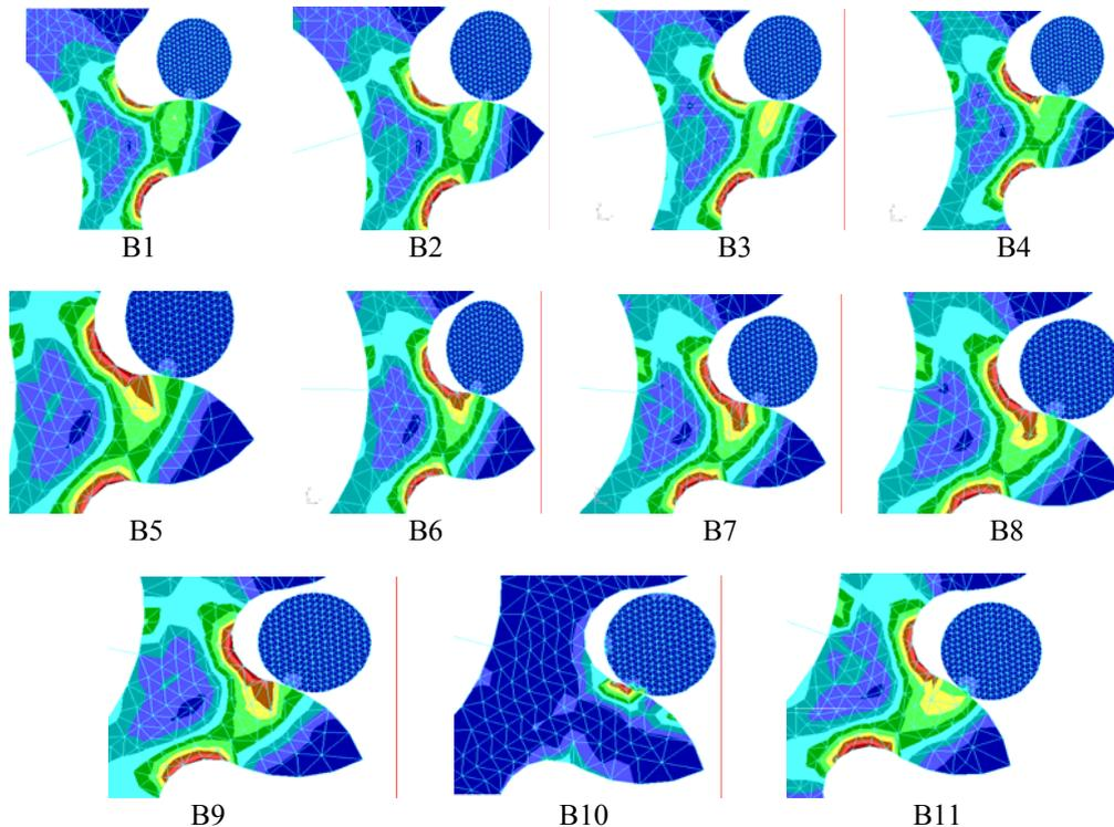
**Fig. 5.** State of tension on the lead wheel at the meshing with the rack pin
