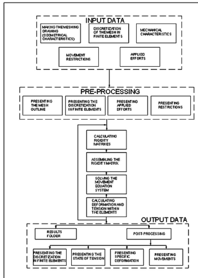
**Fig. 3:** The main stages for solving contact problems
