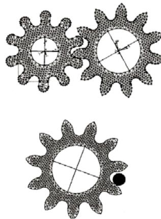
**Fig. 2.** Finite elements modeling of the cycloidal gearwheels
