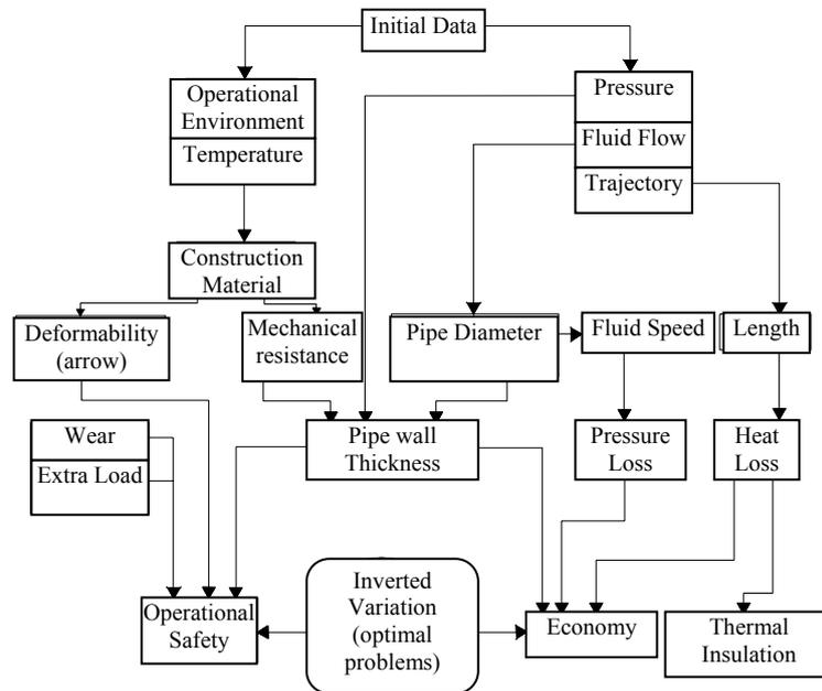
**Fig. 1.** Operational and construction parameters correlation diagram during pipe exploitation and that of material and energy economy
