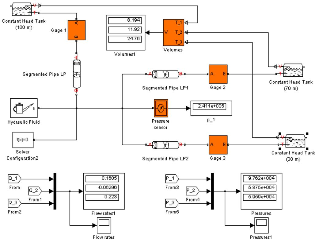
Fig. 4. Free flow simulation model
