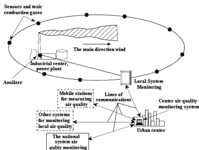
Fig. 4. Schematic diagram of a system for monitoring local air quality near a power plant.
