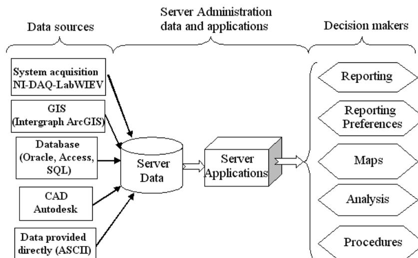
Fig. 1. Block diagram of the integrated information system for environmental monitoring.
