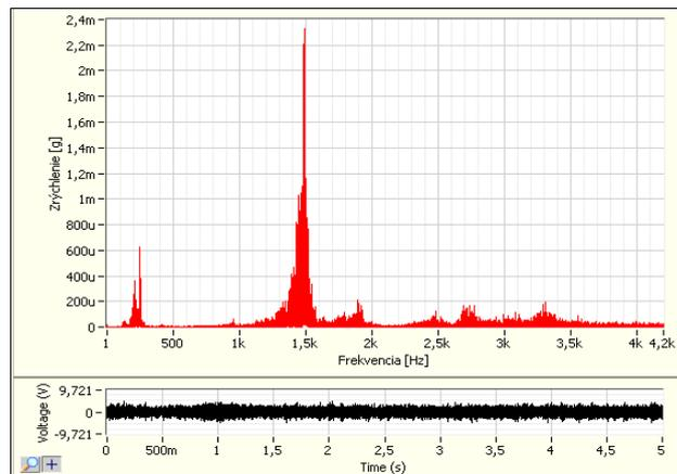
**Fig. 2.** Dependence of vibrations acceleration amplitude course at corresponding frequency on the lineness of abrasive mesh 50 at speed of technological head feed  $50 \text{ mm min}^{-1}$  for the steel S335 JR (11 523)
