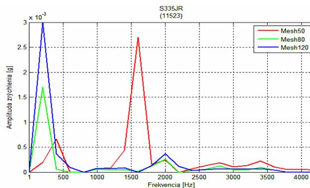
**Fig. 3** Comparing graph of vibrations acceleration amplitude courses at corresponding frequency for three researched dependences of abrasive at speed of technological head feed  $50 \text{ mm} \cdot \text{min}^{-1}$  for the steel S335JR (11 523)
