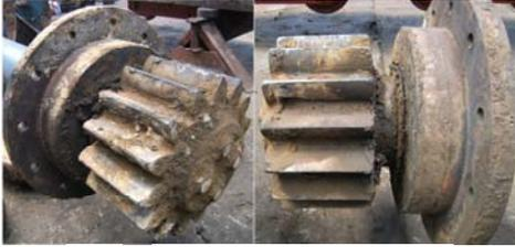
Fig. 8. Wear of the attack pinion
