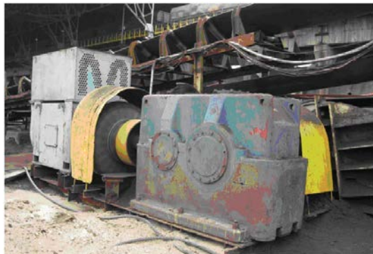
Fig 2. Power electromechanical drive for belt conveyor
