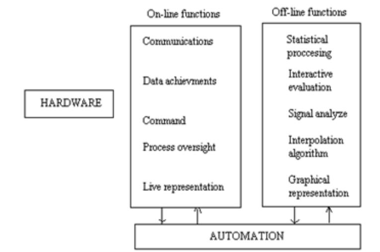
**Fig.3.** The software functions for smart measurements systems
