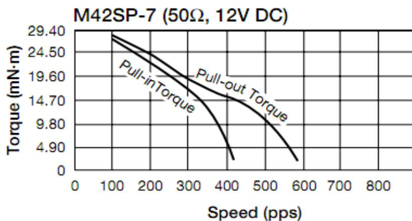
**Fig.1.** Torque/Speed graph
