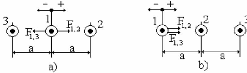
**Fig.3.** Disposition of conductors in the same plane: a) Forces exerted on the median conductors
