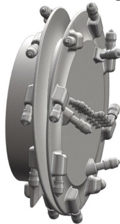
Fig. 7. Cutting organ in the form of a helical drum
