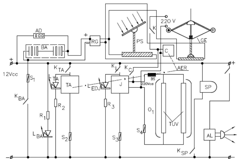
**Fig. 5.** Electrical scheme of the ozonization device
