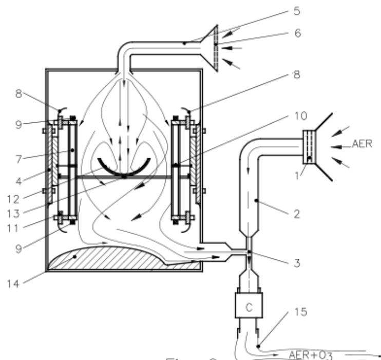
**Fig. 2.** Section through the ozone-generating device
