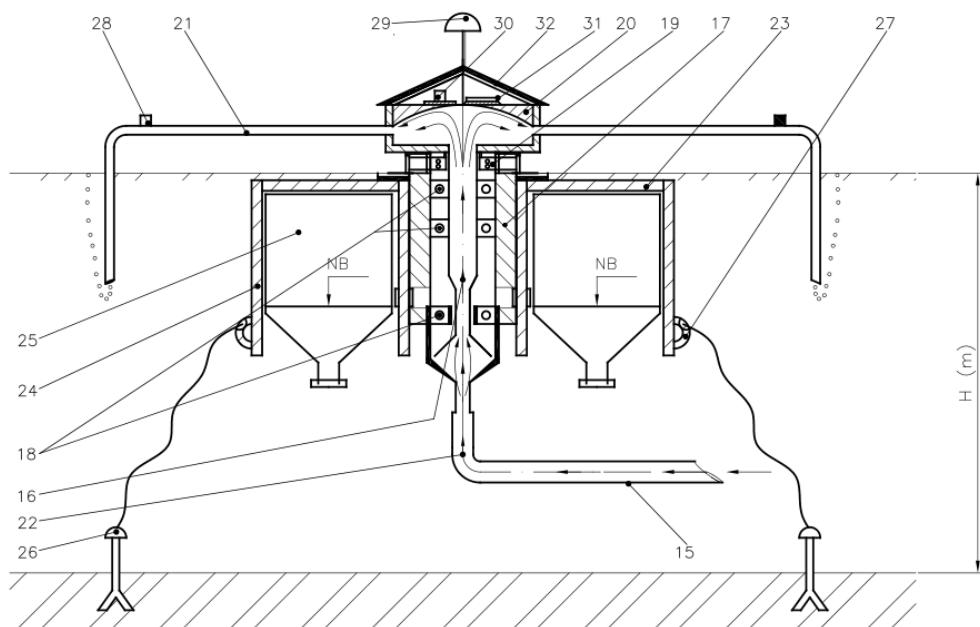
**Fig. 3.** Section through the ozonation device
