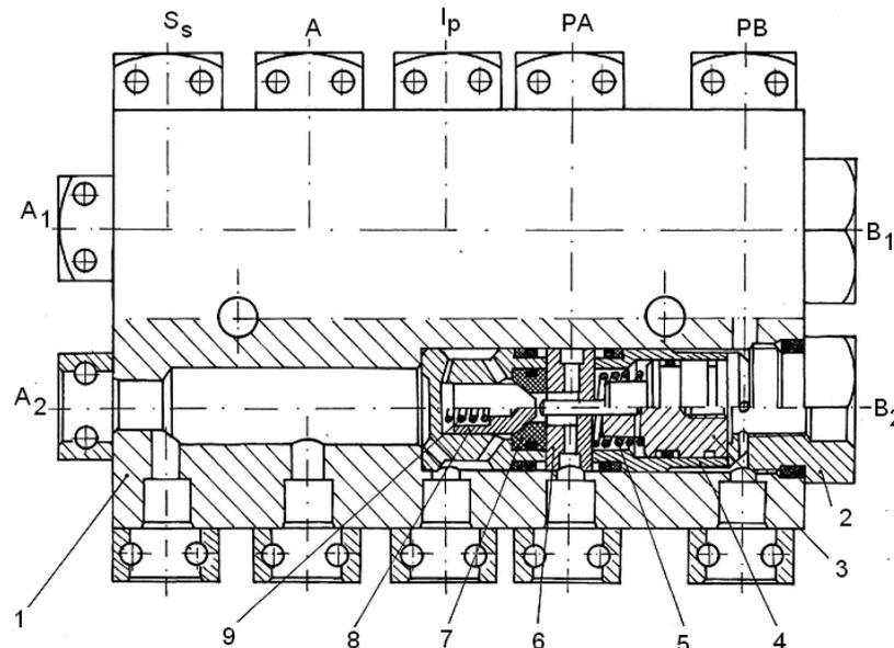
**Fig.8.** Double deblockable valve of direction:
