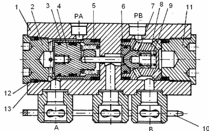
**Fig. 6.** Unblockable direction valve:
