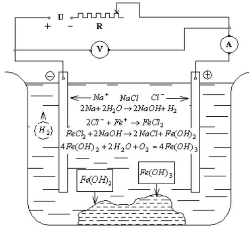
Fig.1. Processing diagram by electrochemical erosion.
