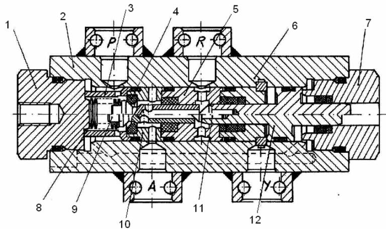
**Fig. 5.** Controlled direction valve normally open:
